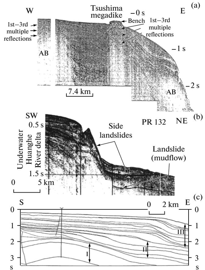
**Fig. 8.** (a) continuous seismic profiling record (Profile 17 across the Tsushima dike [20, 43]); (b) continuous seismic profiling record (Profile 132 across the southern landslide cirque (“bay”) of the Ulylydo Basin); (c) deep CMP section with cross-bedded seismofacies of the underwater Huanghe River delta recovered by the Dolgoran-1 Borehole: (I–III) the sedimentary units dated at 16–12, 12.0–6.5, and 6.5–0 Ma, respectively [18, 37]. For the position of the profiles, see Fig. 6 B.
