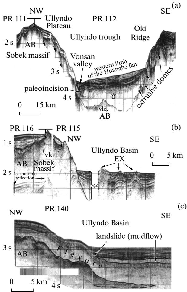
**Fig. 7.** (a–c) continuous seismic profiling records (Institute of Marine Geology and Geophysics, Far East Branch, Russian Academy of Sciences) across the western slope of the Ulylydo Basin and trough [18].
